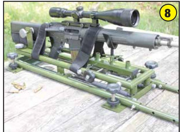
Now that everything is set up, load the gun and fire 1 or 2 shots to seat the gun in the rest, then go back and re-secure straps and vise. You are now ready to begin using the rest. Instructions for mounting the trigger release system are found further along in this booklet.
