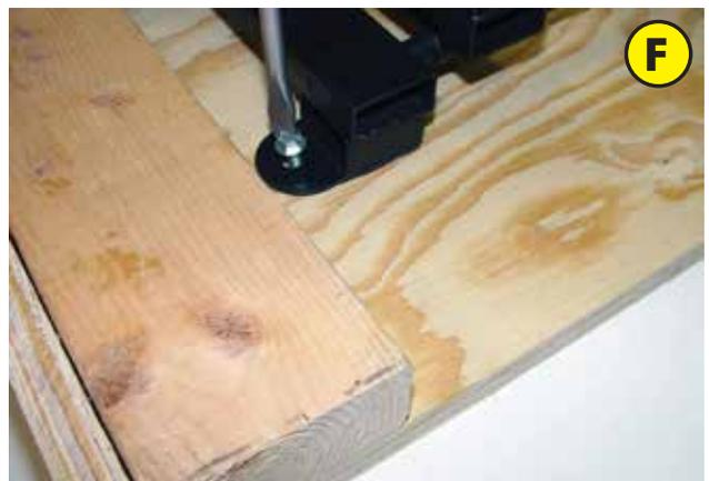
Use 2 - 5/16" X 3/4" sheet metal screws to anchor the left & right sides of the rest. You may find it necessary to stack several flat washers between the flange on the rest and the plywood.
