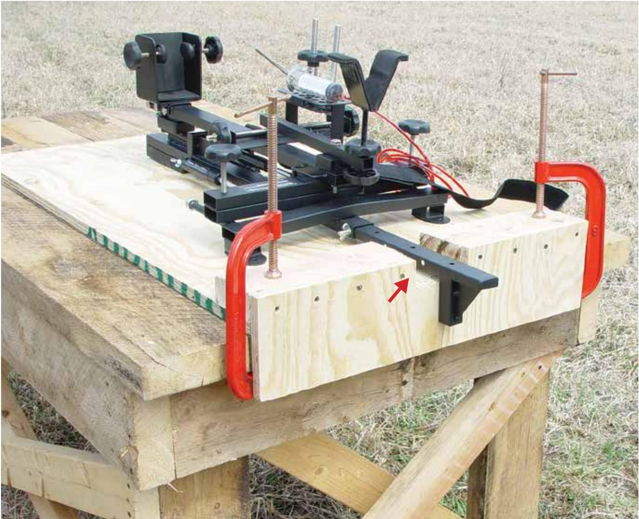
All of the above captioned rifle rests must be secured to a bench. When there is a concrete bench or a range that doesn't allow shooters to screw anything to their benches it is necessary to mount your rest to a platform that can be fixed to the bench using "C" Clamps.
