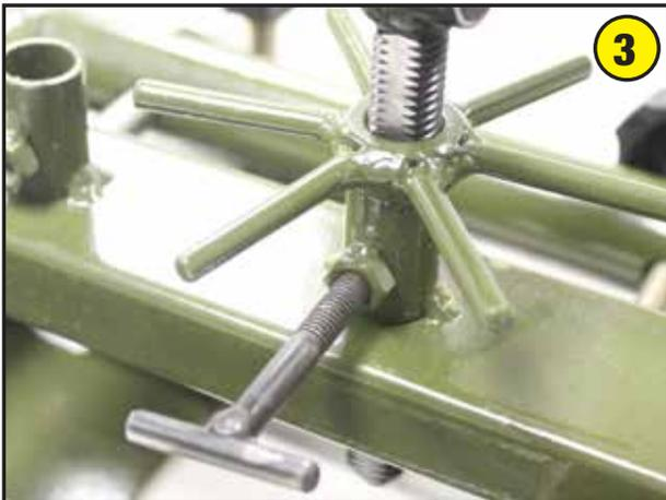
Install the T bolt. The end of the T bolt rides against the flat part of the shaft on the V notch. If you loosen the T bolt too much the shaft will rotate, if you tighten the T bolt so it's making firm contact with the flat side of the shaft and then back it off  $\frac{1}{8}$  of a turn you will be able to operate the capstan knob and this will move the V notch up and down. When you are at your preferred elevation tighten the T bolt and the elevation will remain fixed.
