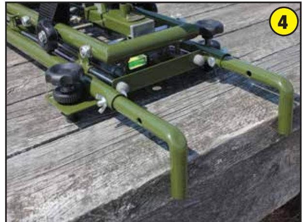
Install the bench grip arms. Simply extend the arms over the end of the bench insert them into the tubes as shown, and secure with the supplied bolts and wing nuts. It is important that these arms firmly grip the forward edge of the bench so that the rest does not move.
