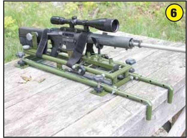
Now that the rest is properly secured to a stable bench, mount the gun in the rest. Firmly place the butt of the gun against the retainer strap and tighten both halves of the vise, just so the gun is secure.
