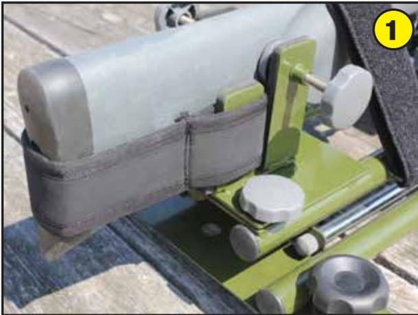
Using the 2 small knobs mount the vise assembly to the rear of the rest as shown. (Vise half forward and the strap retainers to the rear.)
