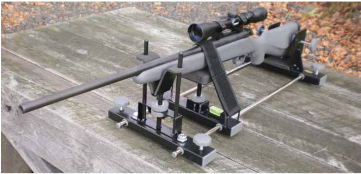
Step 4B: Set the vise in the same location as when you fired. Adjust vise so that reticle is on the + Mark.
