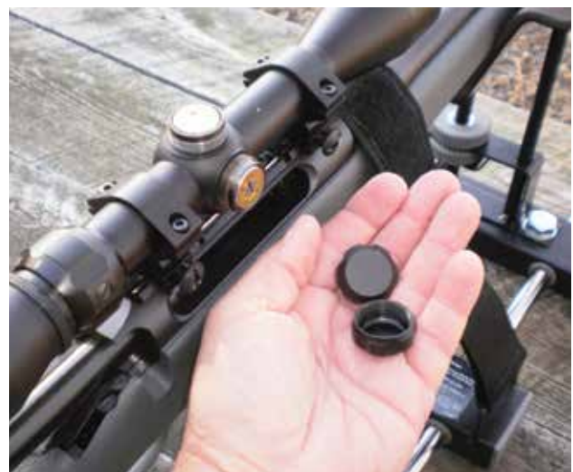
Step 5: Without moving the vise adjust sight until the reticle is on the center of the group.
