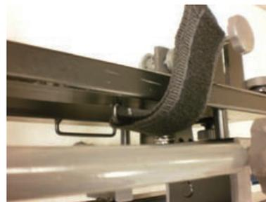
The cleats for the rear strap are on the underside (to avoid making contact with the gun). This is a detail of the easiest way to fit the strap.
