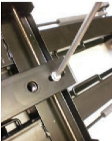
Fit the small round hole in the arm over the threaded post (see 81 Step 2) and fit the slotted hole over the fitting at (C1 in Step 3).
