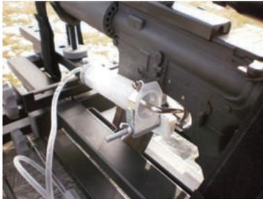
This set includes a remote hydraulic trigger release so that the gun can be fired without human induced motion contamination. Instructions are further on in this book.
