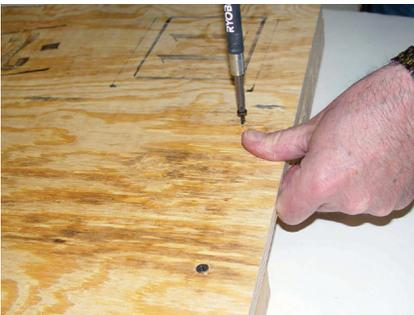
Use 2" screws to secure the 2" x 4" x 10" blocks from the underside.
