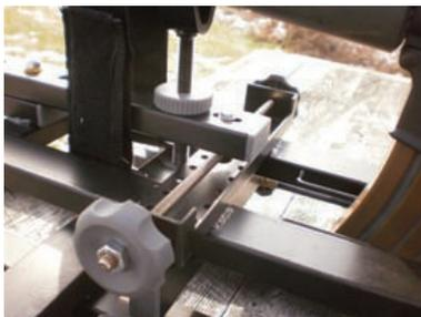
If there is side to side play in the windage adjustment back of the hex nut on one end then tighten the knob to eliminate the play and re-tighten the nut. You may have to do this more than once to eliminate the play but not create binding.
