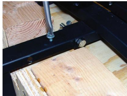
Use 1 - 5/16" x 1 1/2" (or 2") sheet metal screw to anchor the bench grip arm.
