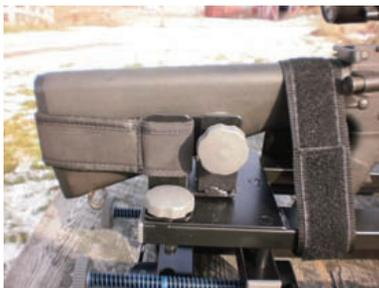
Generally you would use the straps only when testing accuracy and repeatability. This is how the rear strap fits.
