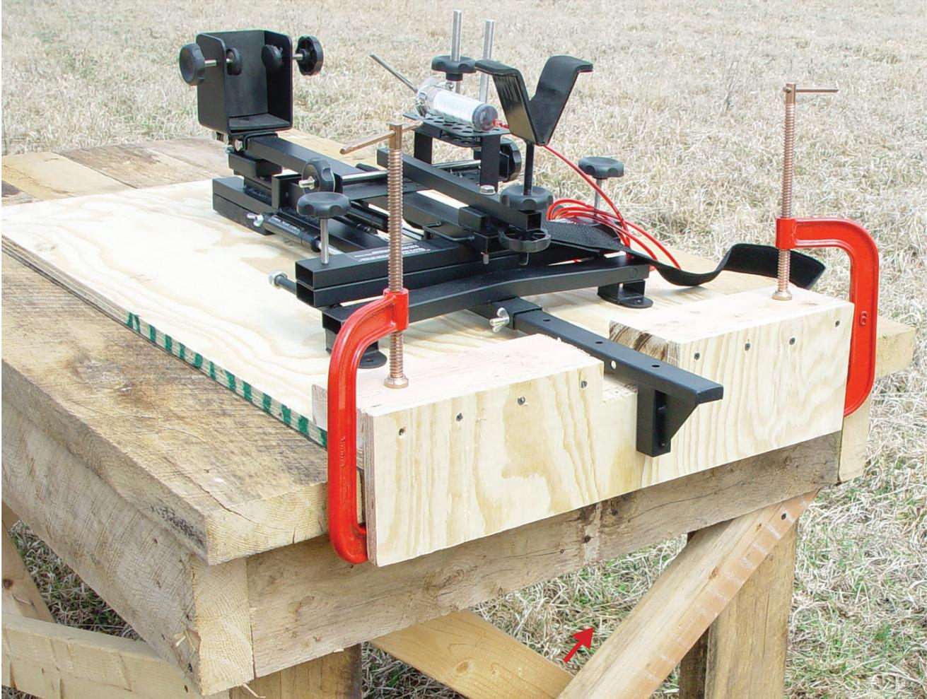
All of the above captioned rifle rests must be secured to a bench. When there is a concrete bench or a range that doesn't allow shooters to screw anything to their benches it is necessary to mount your rest to a platform that can be fixed to the bench using "C" Clamps.
