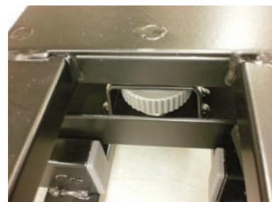
This is the thumb wheel for operating the fine elevation. The best way to use this feature is to put it in its lowest position then count the turns to raise it to maximum height then lower it half the number of turns. This way you will have adjustment in both directions.
