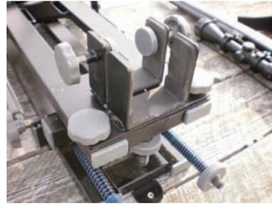
Install the rear gun support & vise assembly as shown. The two small knobs are used to prevent twisting. By using the 2 large (M-16) lock knobs the rear gun support can be used as a secondary elevation adjustment.
