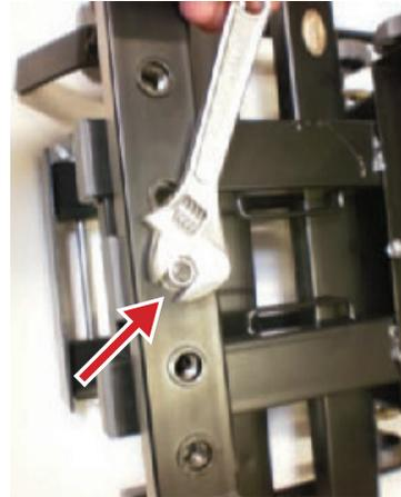
Unscrew the nut. Remove it and the washer.
