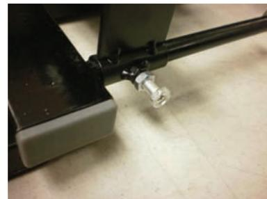
There are two slack adjusters forward and two rear. If there is slack or play between the rails and collars install the adjusters as shown. Back off the hex nut and tighten the screw until it contacts the rail. Now back off the screw ⅛" to ¼" turn and lock in place with the hex nut.
