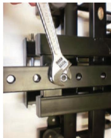
Place the washer over the threaded post and tighten the lock nut (flat side down). Operate the windage knobs. Adjust the nut so that the arm moves freely.
