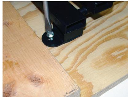
Use 2 - 5/16" x 3/4" sheet metal screws to anchor the left & right sides of the rest. You may find it necessary to stack several flat washers between the flange on the rest and the plywood.
