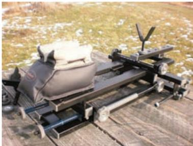
Removing the rear gun support & vise assembly exposes a platform that can be used with rest bags.
