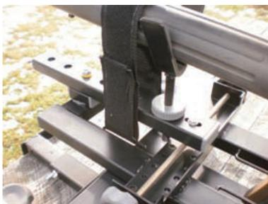
Detail of how a forward strap fits. Note that the rear strap should be tight but the forward straps should allow about 1/4" clearance to allow the barrel to float.
