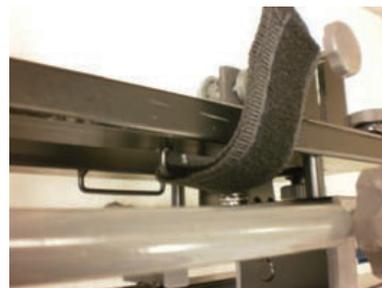
The cleats for the rear strap are on the underside (to avoid making contact with the gun). This is a detail of the easiest way to fit the strap.
