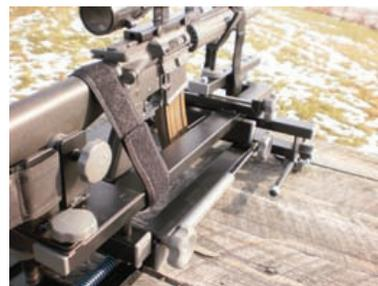
There are 3 pair of cleats for anchoring the Velcro web straps. Only 2 straps are necessary but different gun designs require different locations for the straps. When firing off the shoulder the straps are not necessary.
