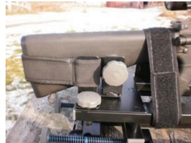
The gun retaining strap installs as shown. Its purpose is to allow the shooter to shoot off the shoulder and use the recoil reduction feature. It also insures that the gun retains its same position in the rest after each shot.
