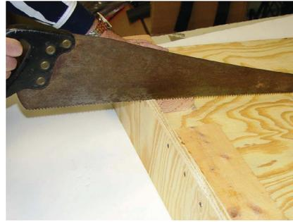
Before cutting the notch examine your rest. Different models require different size notch(es). Notch the front so that the edge of the notch is flush with the surface of the plywood base. This can be done either before or after it is fixed in place.
