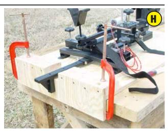
Use 2 or 4 - "C" clamps to anchor the completed set-up to the bench.
