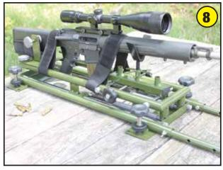
Now that everything is set up, load the gun and fire 1 or 2 shots to seat the gun in the rest, then go back and re-secure straps and vise. You are now ready to begin using the rest. Instructions for mounting the trigger release system are found further along in this booklet.
