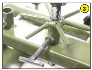
Install the T bolt. The end of the T bolt rides against the flat part of the shaft on the V notch. If you loosen the T bolt too much the shaft will rotate, if you tighten the T bolt so it's making firm contact with the flat side of the shaft and then back it off 1/8 of a turn you will be able to operate the capstan knob and this will move the V notch up and down. When you are at your preferred elevation tighten the T bolt and the elevation will remain fixed.
