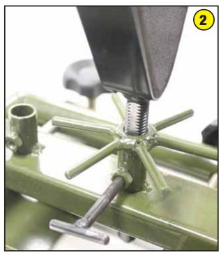
Install the V-notch. Make sure the flat side of the shaft is facing the screw hole for the T bolt.
