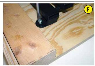
Use 2 - 5/16" X 3/4" sheet metal screws to anchor the left & right sides of the rest.
