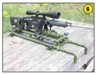
Now that the rest is properly secured to a stable bench, mount the gun in the rest. Firmly place the butt of the gun against the retainer strap and tighten both halves of the vise, just so the gun is secure.
