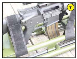
Now use the 2 Velcro straps to secure the gun. The rear strap, which will typically go around the wrist area of the stock, should be firmly and tightly secured. The forward strap is basically a safety strap and therefore, should leave about 1/4" of free play between the strap and the gun so it does not create any bedding related issues.
