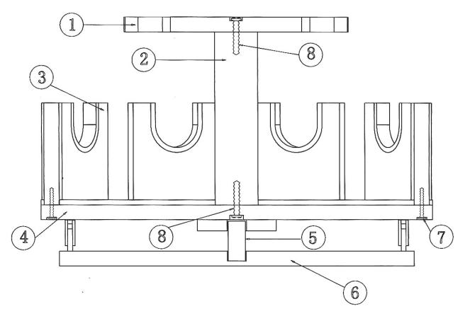
1-2 lbs/ft of torque is sufficient for tightenning the screws.
