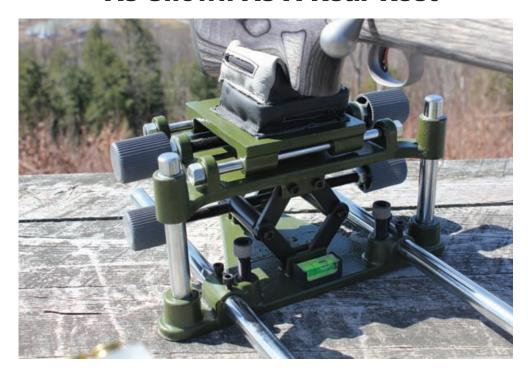
Turn the lower set of knobs to elevate. Turning the upper set of knobs adjusts windage by moving the platform side to side.
