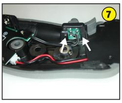
The adjustment that needs to take place is at the right hand corner and left hand face of the plastic clip used to retain the button assembly in place.
