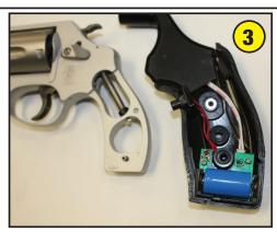
Almost all J Frame revolvers have a referencing / positioning pin towards the butt end of the grip frame. This pin, of course, is used to correctly position the grip halves and it also prevents them from moving during recoil. Both halves of the grip light have a positioning hole with a rubber grommet which is there for the exact same purpose. When installing the grip light each half of the grip must engage the pin on the revolver frame in order to ensure correct position and function.
