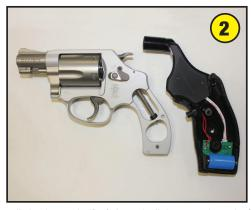
Now install the larger half of the grip light onto the grip frame of the revolver as shown. Please refer to the next step for positioning.
