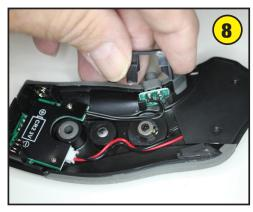
The retainer is mechanically held in place and can easily be removed with the thumbnail and forefinger. Please pay attention to which side is facing out as it is directional and it must be replaced with the same side facing outwards.
