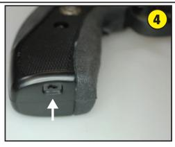
Fit both halves to the gun frame, using the screw provided secure the grip assembly to the gun. Before tightening make sure that there is a flush fit at the seam around the perimeter of the grip. This will indicate that everything is in its proper place. Now tighten the screw until it is snug.
