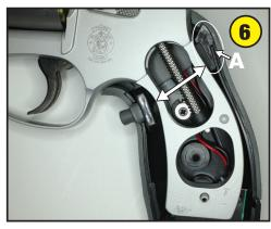
Over the many years that J frames have been manufactured you can rest assured that there have been minor changes in tolerance and dimensions. Therefore, we have manufactured our grip to fit the smallest frame, which means that some frames might be slightly (a few thousandths of an inch) wider at some points. (Note the arrows in the picture.) In that case the grip will appear not to fit. This is easily remedied with minor adjustments.
