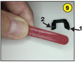
The adjustment is simple. Take a file (an emery board nail file will do) and with the fine side take 3 or 4 strokes on corner #1 and 3 or 4 strokes on face #2 then replace the clip and fit the gun into place. If it is still tight, with slight pressure force the frame of the gun against the recoil bumper (part A in Step #1), and you should be able to get the frame to fit into place. If not, use the file to remove a little bit more material from the clip. This should solve the problem.
