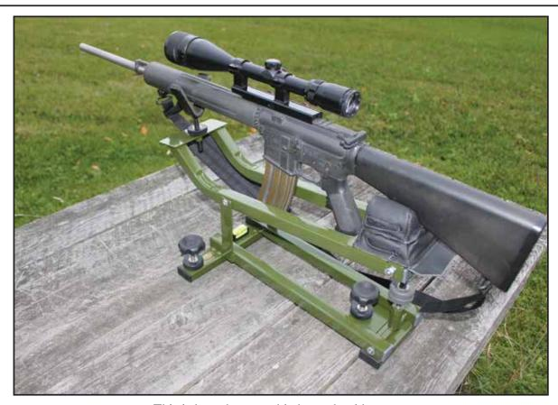
This is how the assembled rest should appear.
