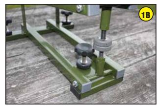
Screw the locking collars onto the levelers and then screw the 3 levelers into their respective threaded holes. The levelers can be used as a secondary elevation adjustment.
