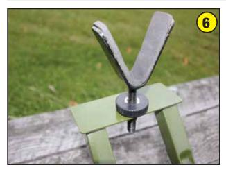
Thread the locking knob into the V notch shaft and thread it into the forward platform. This will serve as the coarse/primary elevation adjustment.
