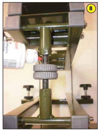
Use acid free machine oil to lubricate the elevation assembly.
