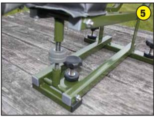
Turn the knob on the elevation assembly so that 7/8'' - 1'' of thread shows above and below the knob. This will put the rest in the middle of the adjustment zone.
