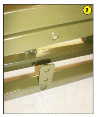
Center the upper assembly of the rest between the 2 support posts. Align the holes in the posts in the upper assembly and thread in 1 shoulder bolt from each side, tighten with a #2 Phillips screwdriver. Tighten enough so that the head of the bolt is flush with the support post, but not so tight that you create binding.
