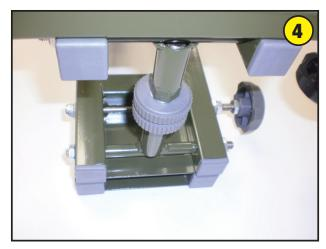
Turn the rest over and attach the other end of the elevation assembly using the other 6" bolt and hex nut as shown.
