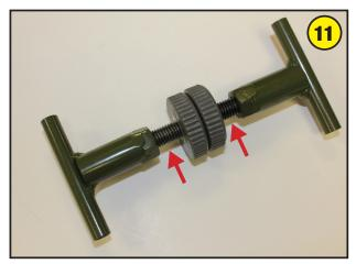
Operation - Before attempting to elevate the rest operate the knob on the elevation assembly so that approximately 1" of thread is showing above and below the knob. This will put you in the middle of the elevation range. In other words, now you'll be able to move the elevation both up and down. Fix the forward leather rest bag to the front support, place the rear rest bag on the rear platform.
