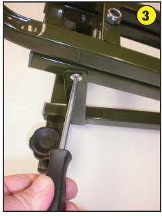
Center the upper rest assembly between the uprights in the lower assembly, align the holes as shown and attach with 1 shoulder bolt from each side. Tighten until snug, but not too tight that the rest binds.
