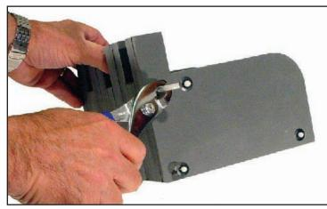
2. Using 3/18" threaded rods, nuts and washers (purchased separately) assemble as many sections together as necessary.
