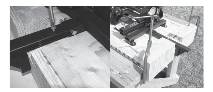
Use 1 - 5/16" x 1 1/2" (or 2") sheet metal screw to anchor the bench grip arm.
