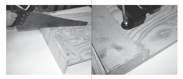
Notch the front brace so that the edge of the notch is flush with the surface of the plywood base. This can be done either before or after it is fixed in place.
